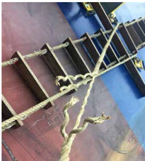
Example of an unsafe man rope.
