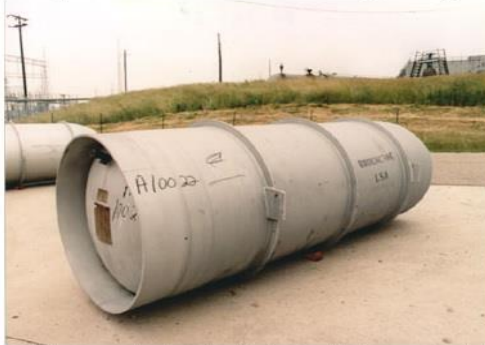
After enrichment, depleted uranium hexafluoride is placed in large steel cylinders for storage. The most common storage cylinders have a 48 inch diameter.
